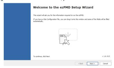
Drag the provided site-specific configuration XML file onto the central area of this screen and press Next.
